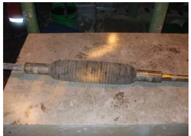
Inflatable packer showing fixed head (left), inflated gland and sliding head (right)
