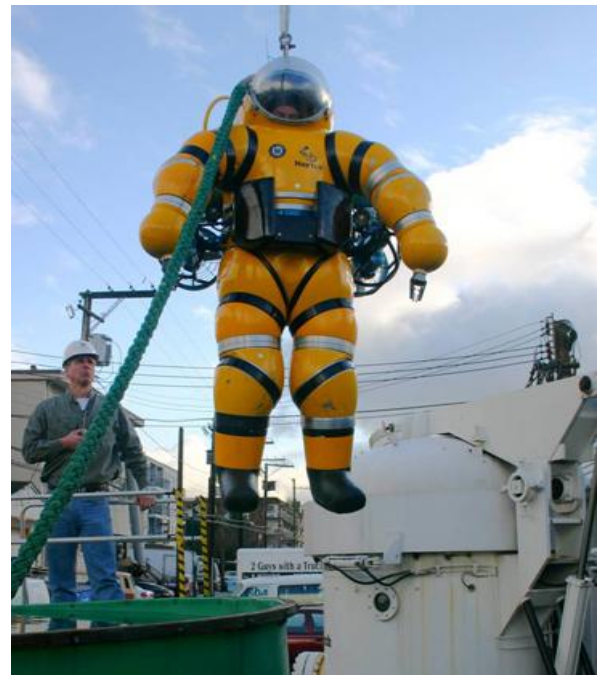
Specialized atmospheric diving suits used during the underwater diving operation
